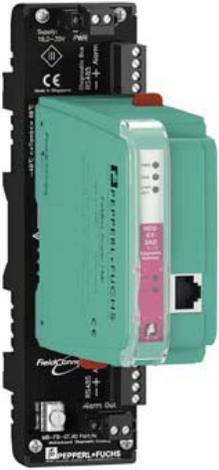
Pepperl+Fuchs FieldConnex diagnostic gateway significantly enhances interoperation between individual advanced diagnostic modules (ADM) of a fieldbus infrastructure and the diagnostic manager in the control room by allowing information to be exchanged in both directions via Ethernet and enabling additional features such as remote setup of ADMs. ADMs monitor the quality of fieldbus communication for FOUNDATION fieldbus H1 and Profibus PA networks.
