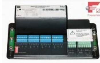
Extensive function block support ensures that such solutions benefit from particularly powerful FOUNDATION fieldbus technology features. The coupler provides DI, DO, MDI, and MDO functions, and advanced functions such as AI for frequency signals, CI for counters, and logic transducer blocks for logical input/output combinations.
