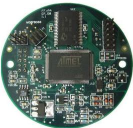
With Microcyber's Fieldbus OEM Solution, users can upgrade FOUNDATION fieldbus devices quickly and easily. The newly designed FOUNDATION fieldbus H1 communication boards are customized to meet specific requirements, allowing the upgrade of traditional instruments to FOUNDATION fieldbus devices quickly. The boards include a stack, function blocks, communication circuit, and interface circuit.
