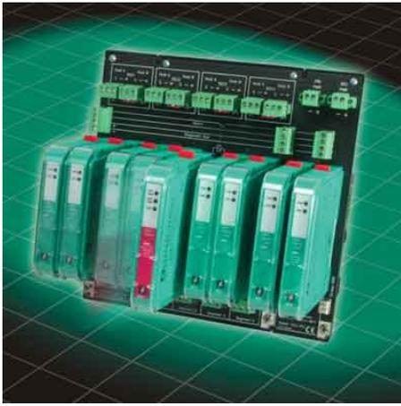
relay output," says Brian Traczyk, product manager, Pepperl+Fuchs. "The user simply sets the signal, noise, and jitter warning levels via easily accessible DIP-switches, with no software required. After the DIP-switches are set, the user just plugs the module into the motherboard to initiate physical layer monitoring. Any warnings will cause a summary alarm via voltage-free contact at the fault output on the motherboard."
