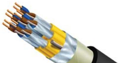
Northwire’s DataCell FOUNDATION fieldbus M-EZ (Marshal-EZ) cables enable fast, simple installation into marshaling cabinets without shrink tubing. They are engineered with up to 24 individually foil-shielded pairs that have an extruded PVC binder over each pair—all contained within a single cable.
