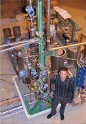
Emerson Process Management's PlantWeb digital plant architecture, incorporating FOUNDATION fieldbus technology, WirelessHART, and Wi-Fi, is being used to automate a pilot ethanol processing plant built by Chematur Engineering AB.
