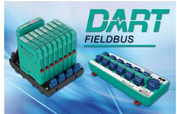
During normal operation, a DART power supply feeds full nominal power of 8 to 50 W, exponentially more power than the approximately 2 W normally permitted in intrinsic safety environments. Should a fault occur, the potential spark remains non-incendive. DART detects the resulting change in current and immediately switches off the power supply. In microseconds, energy from the electrical system is reduced to a safe level, robbing a spark of the energy needed to ignite hazardous gases.
